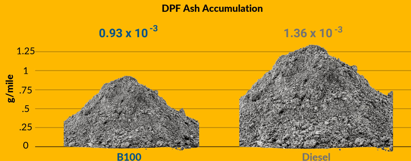
Figure 6 DPF Ash Accumulation (g/mile) Comparison
