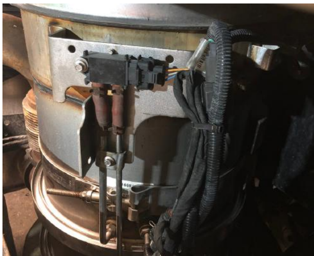
Diesel Particulate Filter Equipped with Monitoring Sensor
