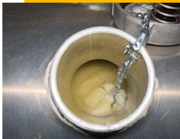
Gelled B100 In Fuel Tank Prior to Vector System Conditioning
